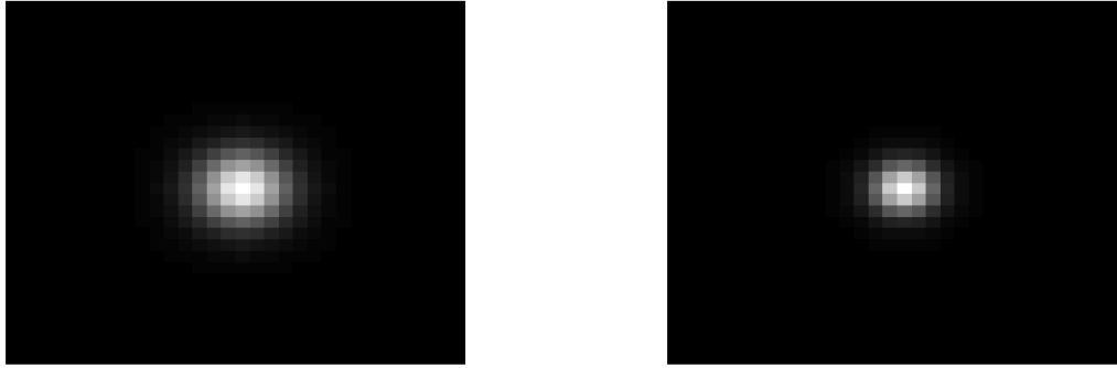
Figure 38. Point spread functions used to generate simulated data and conduct spatial correlation testing. Scenario 1: PSF with r_0 = 5 cm (left side). Scenario 2: PSF with r_0 = 8 cm (right side).
